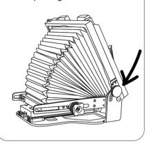
(5) Screw front standard into desired base mount (see page 10 for guidance).
